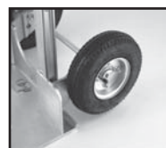
D9 8" x 2.5" Pneumatic 2 pc. Steel Hub 500 lb. Capacity
