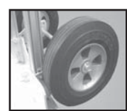
D2 10" x 2.5" Semi-Pneumatic 1 pc. Plastic Hub 500 lb. Capacity
