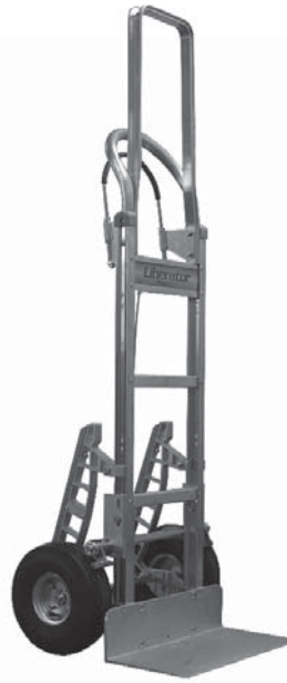
A1-B1-C6-D5-E1L-E60-BTC Standard loop handle, frame extension for 60" overall height, 18" x 9" extruded aluminum noseplate, tread brake technology for food service drivers, 600 lb capacity
