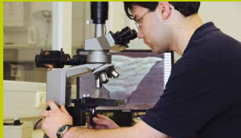
Microscopic weld seam inspection
