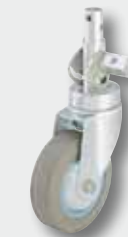
Swivel castor with central wheel and swivel head brake, directional lock, special swivel head bearing and non-marking tyre.
