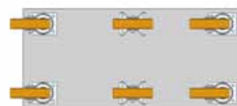
Four swivel and two fixed castors of identical mounting height
