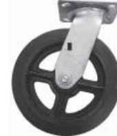
Caster Kit 820 8" Cast Iron Core Mold on Rubber Square Tread (provides 2,500 lb cap.) add -820 to model #
