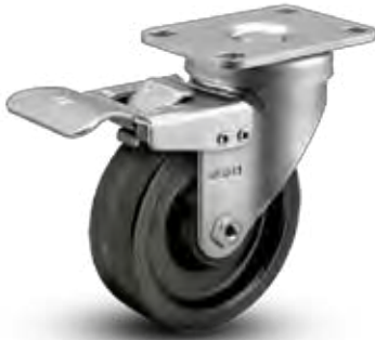
Total Lock Brake Available on O2 Series. Locks wheel and swivel with simple press of toe lever. Specify T .
